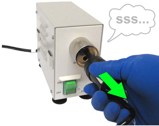
Figure 5. Endoscope being properly depressurized.
