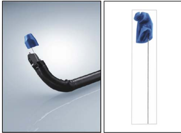
FIG. 19.3 KARL STORZ has designed a duodenoscope with an Albarra Module, a single-use (removable and disposable) elevator wire and forceps. This module importantly facilitates reprocessing by removing a component that is commonly difficult to clean. Image courtesy of KARL STORZ.
