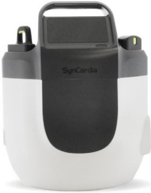
FIGURE 1.11 Appearance models are used in the third formative study to obtain users' feedback about the size, shape, and the location of batteries, handles, and driveline ports.
