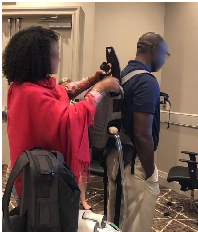
FIGURE 1.15 A former patient and his caregiver replace the batteries in the prototype driver in formative study 4.
