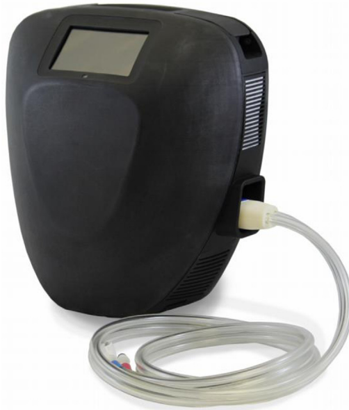
FIGURE 1.14 The functional prototype that contained working pump mechanism, a touchscreen graphical user interface, and alarm sounds and messages.
